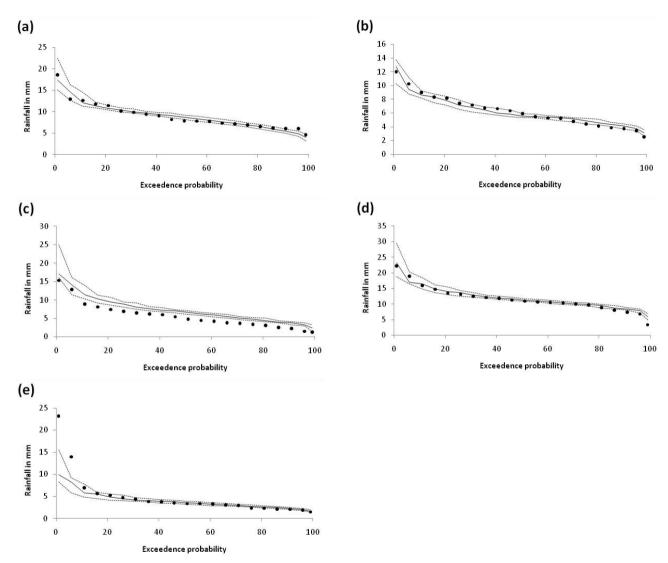
Figure 3.8: 6-minute annual maximum rainfall against exceedance probability for (a) Sydney, (b) Perth, (c) Alice Springs, (d) Cairns, and (e) Hobart. Black dots represents observed data, black solid line represents the median of 100 simulations, and black dotted lines represent the 5
