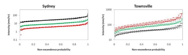
Figure A10: Method of fragments 1, 6 & 24 hr Intensity-Frequency-Duration curves
