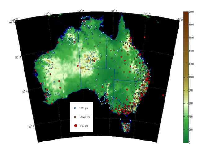
Figure 3.1: Spatial coverage and record length of the Australian sub-daily pluviograph record. Figure extracted from [Westra et al., 2012].
