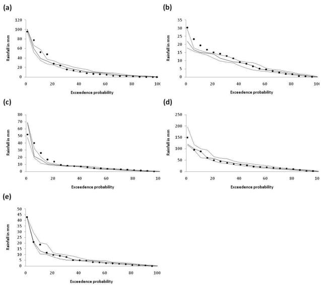
Figure 2.4: 6-hour antecedent rainfall prior to the 6-minute annual maximum storm burst plotted against exceedance probability for (a) Sydney, (b) Perth, (c) Alice Springs, (d) Cairns, and (e) Hobart. Black dots represents observed data, black solid line represents the median of 100 simulations, and black dotted lines represent the 5 and 95 percentile simulated values. Figure extracted from [Westra et al., 2012].
